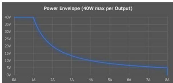
At lower output voltages the power is restricted by the maximum 8A hardware current limit.
