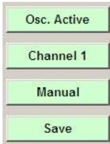
**Osc. Active/Passive:** Activates oscilloscope or shows latest screen display.
