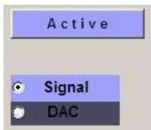
**Active/Passive:** If active, then gives square wave or analogue output from Channel2.
