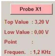
**ProbeX1:** Adjusts voltage value according to X1 or X10 coefficient probe.
